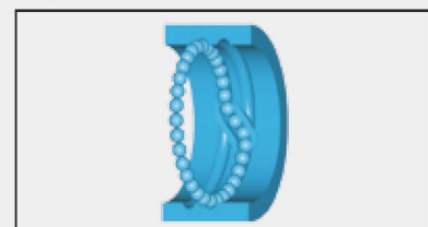
Fig 3.6 Circuit for internal return cap
